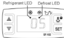
It is a mini-sized and integrated intelligent controller and applicable to the compressor of one Hp.
