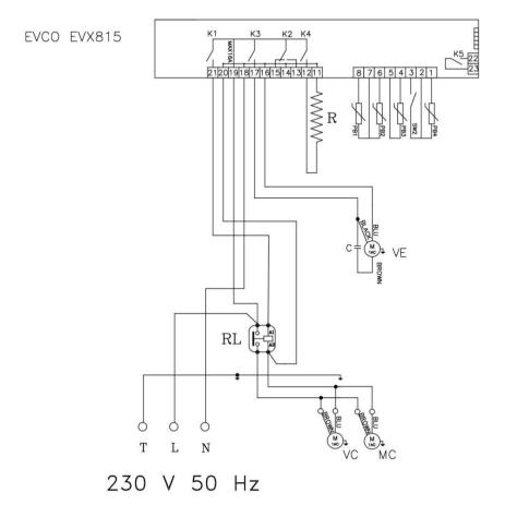
MC: Compressor VC: Condenser fan VE: Evaporator fan 1 RL: Relé 30A C: Condenser 2mf K1: Compressor relay K2: Defrosting relay K3: Evaporator fan relay K4: Heating resistance relay PB1: Pin probe PB2: Cold room probe PB3: Condensator probe PB4: Evaporator probe SW2: Door micro switch
