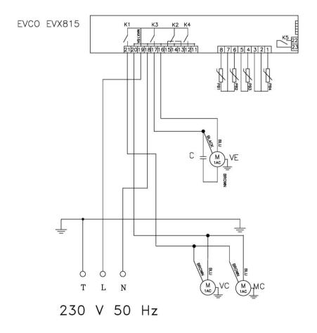
MC: Compressor VC: Condenser fan VE: Evaporator fan 1 C: Condenser 2mf K1: Compressor relay K2: Defrosting relay K3: Evaporator fan relay K4: Heating resistance relay PB1: Room probe PB2: Pin probe PB3: Evaporat. probe PB4: Condensator probe
