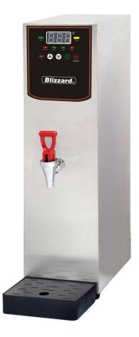
Using conditions: Applicable water source: applicable for municipal water or other potable water, PH between 6.5~8.5, from a <u>filtered Soft water supply</u> Enter water pressure:  $0.2\sim0.4$ Mpa (Rate of flow $\geq$ 4L/min) Enter water temperature:  $0\sim40^{\circ}$ C Input voltage:  $\sim220-240V\pm10\%$ Humidity:  $10\sim60\%$  (non condensing) Ambient temperature:  $5\sim40^{\circ}$ C
