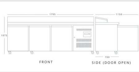
BLIZZARD HBC3EN H 1075mm W 1795mm D 700mm
