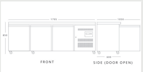
BLIZZARD HBC3SL H 850mm W 1795mm D 600mm
